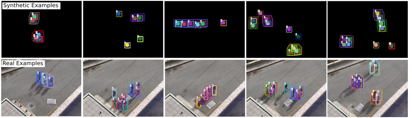
Fig. 2: Some examples of the scenarios contained in the Friends Meet dataset (synthetic and real videos) with the ground truth of individuals and groups.
